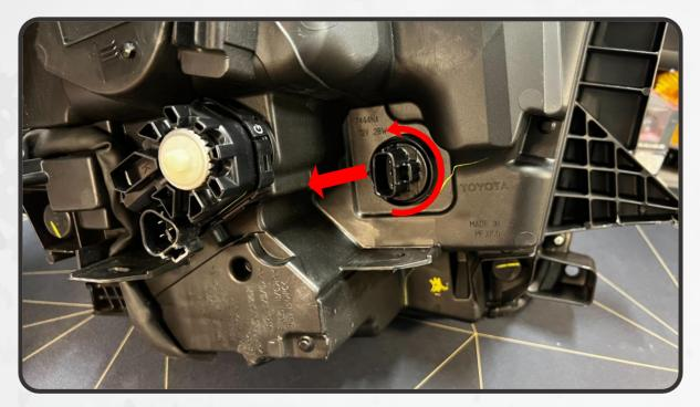
2. REMOVE THE OLD BULB FROM THE TURN SIGNAL SOCKET
