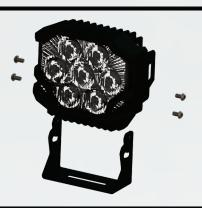
When reinstalling the M6 screws, do not use a power tool and do not overtighten!
