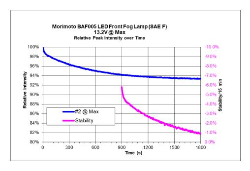
Sample required 20+ minute stabilization period (<3%/15 min).
