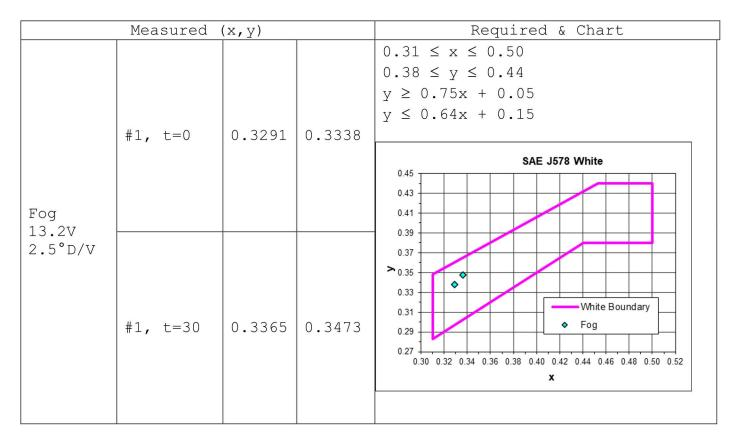
The color of the light emitted through the clear lens falls within the acceptable limits for white at all times.
