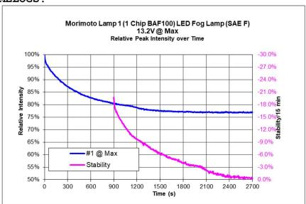
Sample required 30+ minute stabilization period (<3%/15 min).
