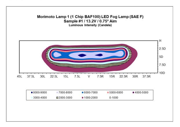
Applied Voltage: 13.20V / 1.098A after stabilization warmup Multiply above values by 1.231 to acquire t = 1 minute values.
