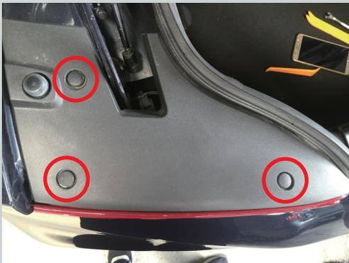
5. Remove the three (3) 8mm nuts holding the tail light to the vehicle.
