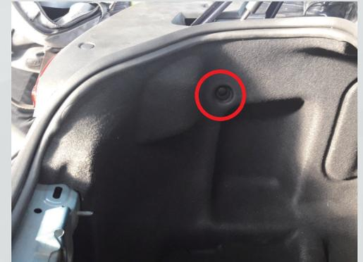
4. Remove the clips securing the trim panel on top of the tail lights. Remove the board and set aside.
