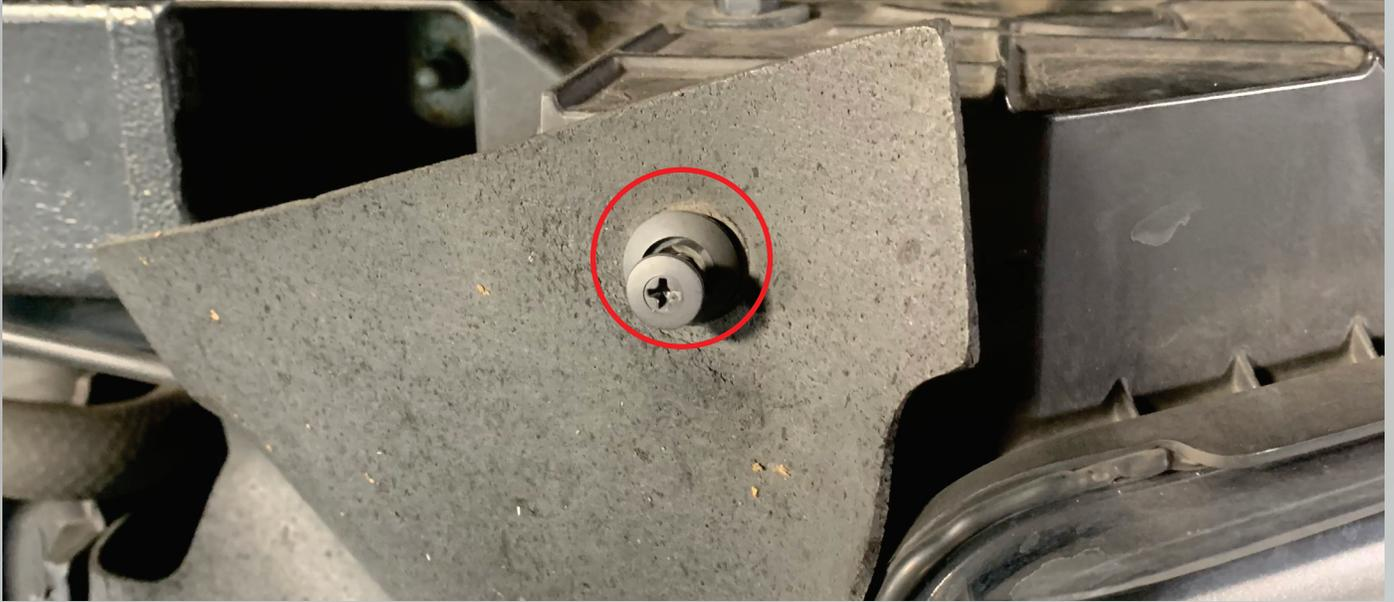
2. Remove the 10mm bolt retaining each headlight behind the grille surround.
