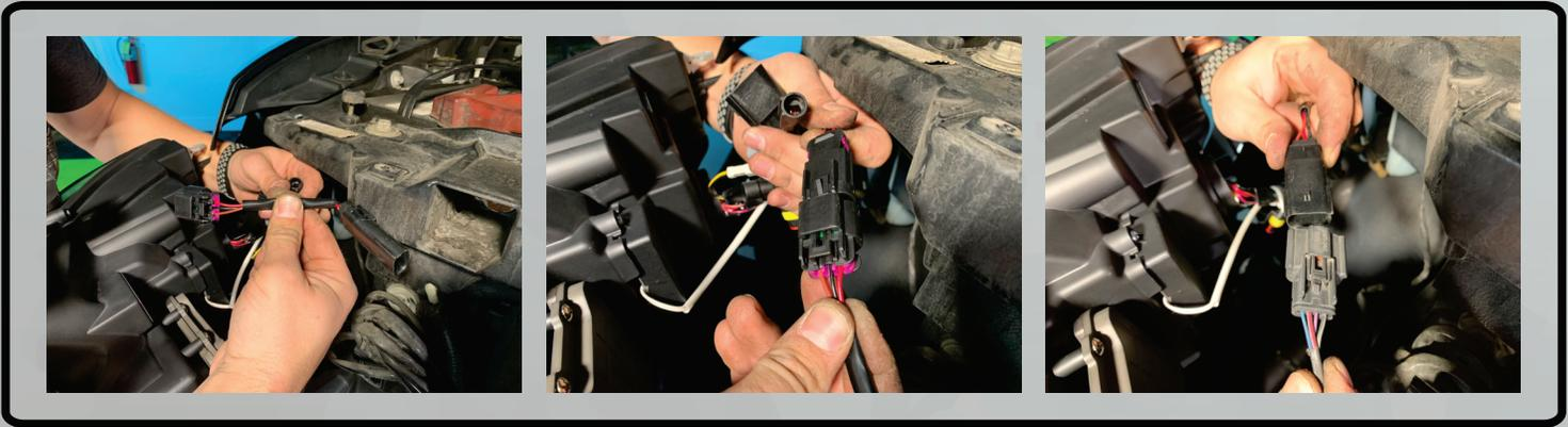
8. Connect the turn signal connector to the factory turn signal plug.
