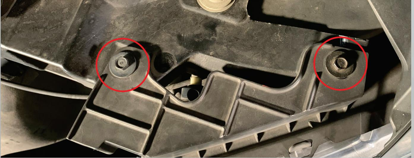
4. Using a trim tool, pop the headlight's ball joint out of the fender clip near the side reflector.
