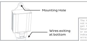
The harness' control box itself does not need to be grounded nor does it get hot enough to melt plastics. Secure it by hanging it from a new or existing bolt or screw from the indicated mounting hole so that the wires exit at the bottom. This minimizes the chance of water ingress.
